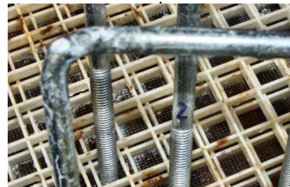
Example of Salt Spray Test to White on Clear Zinc Plating
